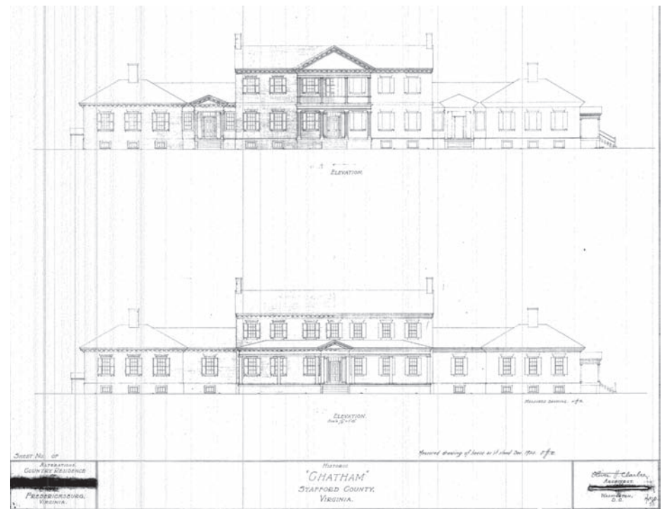
Fig. G: Oliver H. Clarke's 1920 elevation drawing of the west and east sides of Chatham depicting Chatham's Greek Revival porches. (National Park Service).
